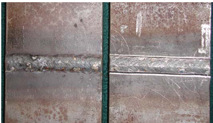
Fig.5. The view of the butt welds in as-welded condition (left side sample) and after application of UP (right side sample) [7]
