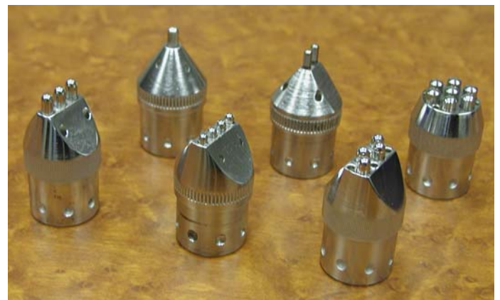
Fig.2. A set of interchangeable working heads for UIT/UP [7]
