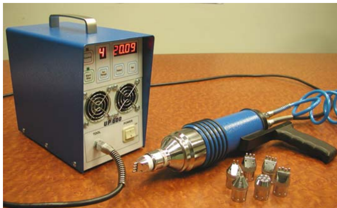
Fig.1a. Basic ultrasonic peening system for fatigue life improvement of welded elements and structures [6]
