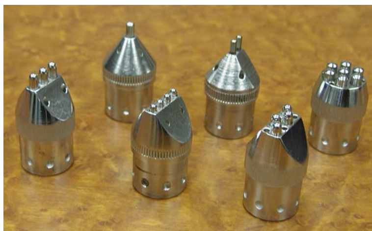
Figure 2. A set of interchangeable working heads for UP
