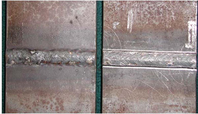
Figure 5. The view of the butt welds in as-welded condition (left side sample) and after application of UP (right side sample)
