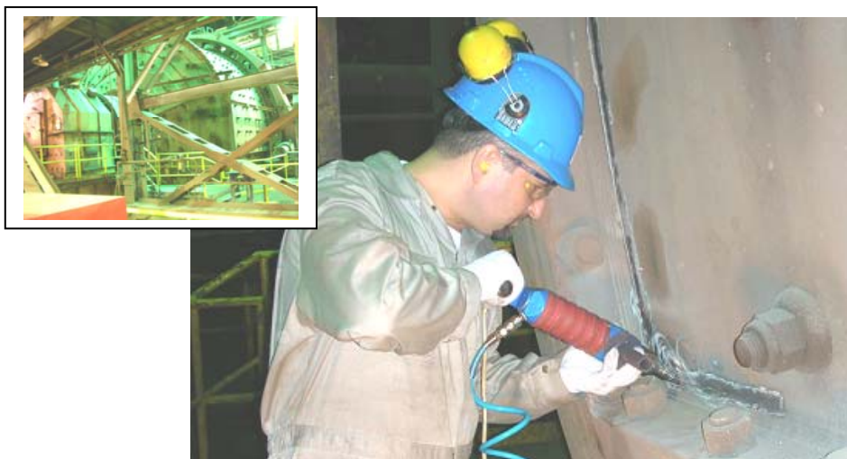
Figure 16. Application of UP for rehabilitation of welded elements of a large grinding mill
