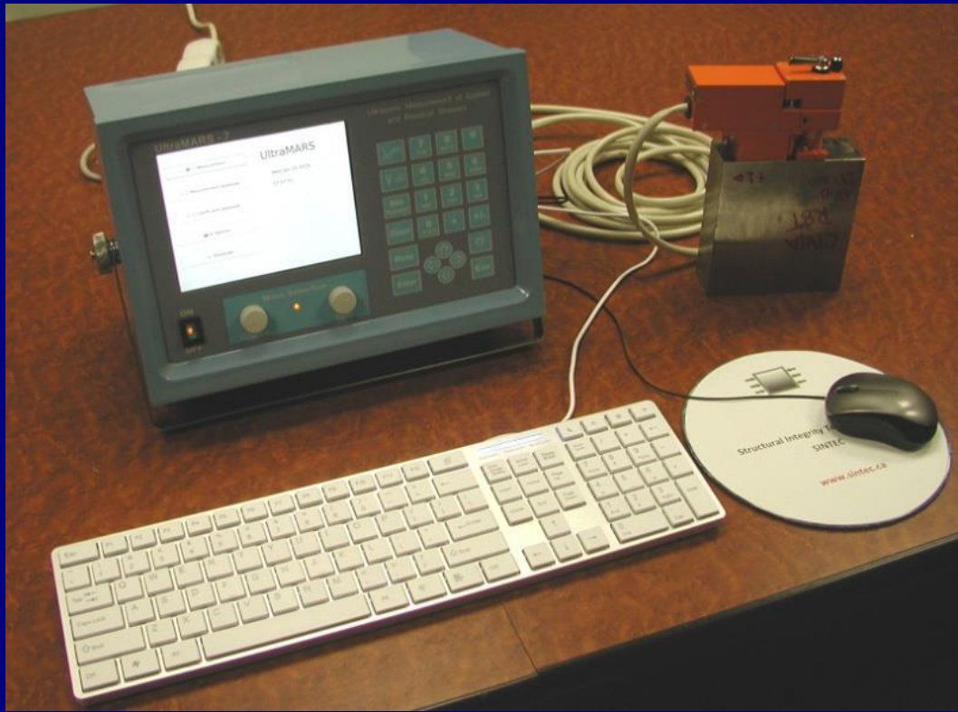
The Ultrasonic Computerized Complex UltraMARS-7 for measurement of residual and applied stresses
