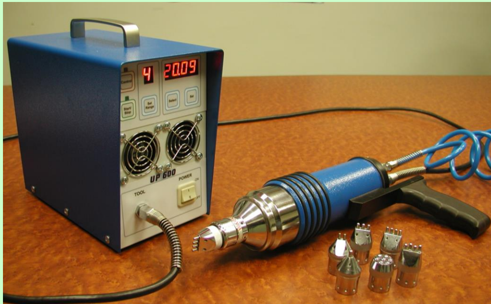
Basic UP system for fatigue life improvement of parts and welded elements
