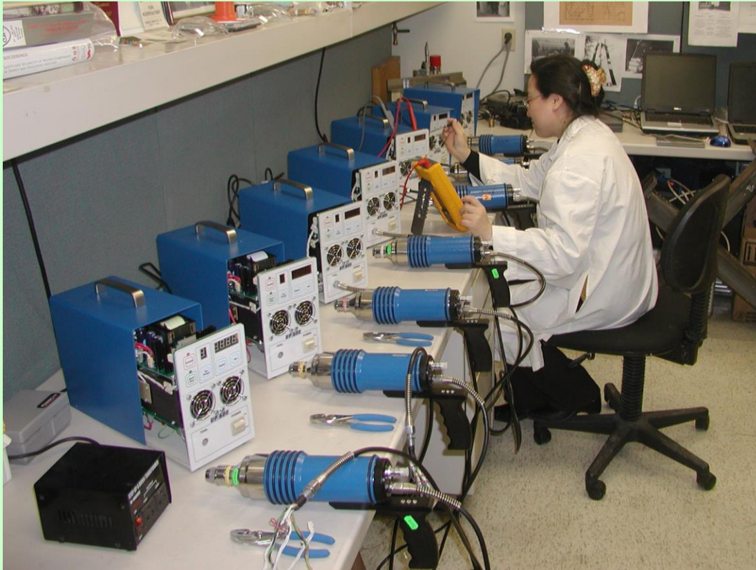
Final assembly and tuning of UIT/UP systems at SINTEC
