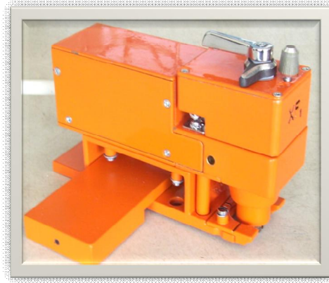
Figure 86 The Mechanical Holder with Transducer Installed
