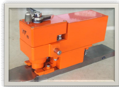
Figure 87 The Magnet Holder with Transducer Installed
